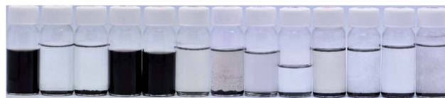
Fig. 3 Photograph of 0.01 wt% GONRs dispersions in various organic solvents 24 h after the ultrasonication treatment (from left: water, methanol, ethanol, DMF, NMP, acetone, THF, MMA, chloroform, styrene, xylene, toluene, hexane).
