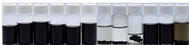
Fig. 6 Photograph of 0.01 wt% CR-GONRs dispersions 24 h after the ultrasonication treatment in various organic solvents (from left: water, methanol, ethanol, DMF, NMP, acetone, THF, MMA, chloroform, styrene, xylene, toluene).
